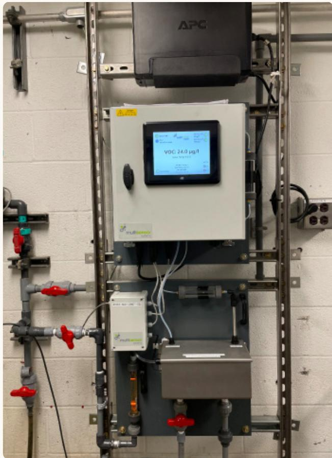
**MS1200 Touch installed on a frame; flow regulation at the intake is of paramount importance to avoid flooding of the system.**
