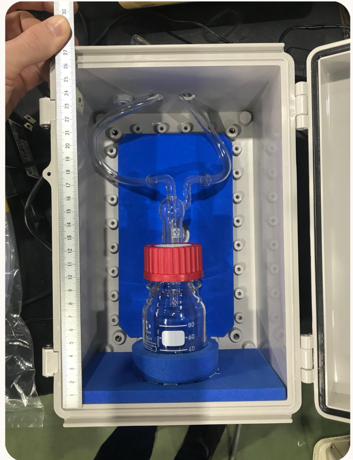
Condensation trap developed by Daiki to ensure the removal of droplets from the gas coming out from the process at high temperature.
