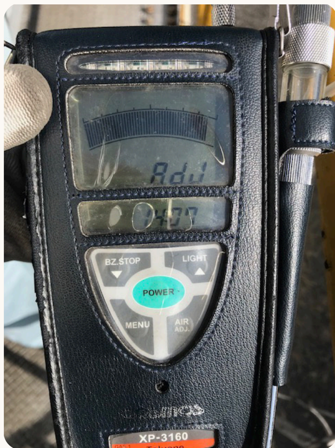
The handheld device used for spot sampling of VOC concentration is not suited for process optimisation and continuous monitoring.
